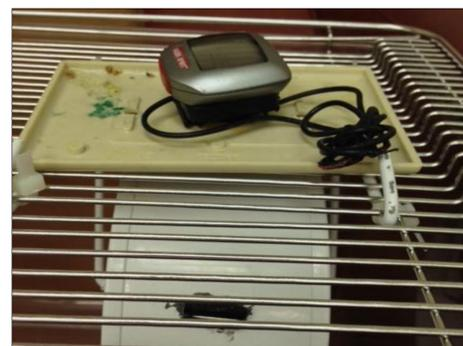
Figure 2: Cage set up including running wheel, magnetic sensor, and digital odometer.
